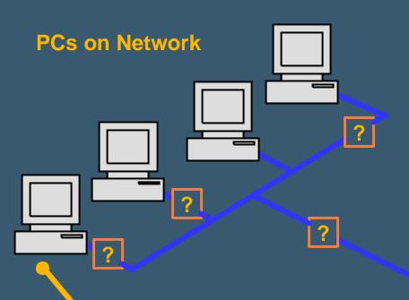
**Discover:** Intel® AMT downloads HW & SW asset information from the BIOS and OS into non-volatile memory during boot, which can be accessed by IT anytime because users can't remove or prevent IT access to the information.
