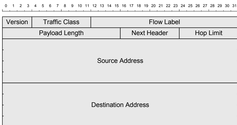
Figure 5 – IPv6 Header
