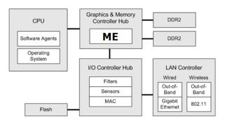
Figure 1: Functional location of one instance of Intel AMT's Manageability Engine (ME).
